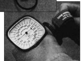
A small probe is placed over a peripheral artery (e.g., digital or coccygeal). An ultrasonic crystal in the probe transmits pulse wave sounds back to the amplifier. The pressure cuff is then placed proximal to the probe. The cuff is inflated until the pulse sounds are no longer audible. The cuff is slowly deflated, using the manometer, until pulse sounds are audible once more, at which point the manometer displays a numeric value of the animal's systolic pressure.
