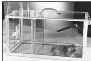
The Lexan anesthesia chamber provides a simple method of induction. Chamber induction reduces restraint, minimizing stress and reducing the chance of injury to the operator and animal. The divider system allows three different size chambers within the one unit: 18"  $\times$  9"  $\times$  9", 12"  $\times$  9"  $\times$  9", and 6"  $\times$  9"  $\times$  9". 10 lbs.
